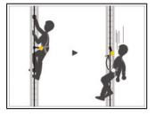
The textile dorsal attachment point allows connection of a self-retracting fall-arrest system.
